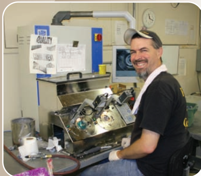
Hand blocking the 15 to 20 pairs of glass lenses a day is Rod Leidy.
